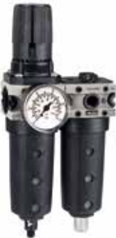
Filter/Regulator + Lubricator Combinations (50mg/m³) 5 micron element, 8 bar Regulator + Gauge and Wall Mounting Brackets
